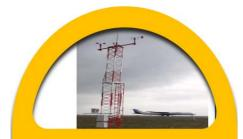
**2021:** Current Weather Instruments System (CWIS) on frangible mast installed at Tirupati airport.
