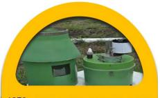
**1970:** Self-recording raingages (SRRG) record the rainfall depth in the form of a continuous plot.
