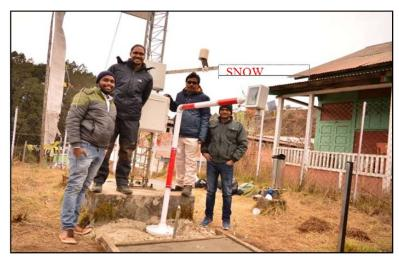
Snow Sensor installed at Tawang, Arunachal Pradesh
