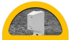
**1974:** Ceilometer was installed to estimate the height of the base of the low clouds at Mumbai.
