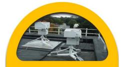
**1990:** First vertical distribution of atmospheric column ozone using Brewer spectrophotometer.
