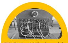
1882:A Telephone Switchboard was a device used to connect circuits of telephones to establish telephone calls between users or other switchboards.
