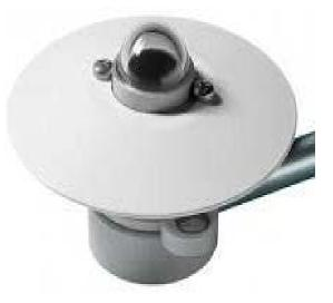
The sensor uses a thermocouple constantan junction. А copper Thermo junction is created on top and bottom surface. The Top surface is coated with optically black paint for absorbing 98% of solar Radiation with reference to black body. The Top surface absorbs solar Radiation and acts as a hot junction. The bottom surface in shadow acts as a cold junction. A hemispherical glass dome on the sensor allow only short wave Radiation coming from Sun.
