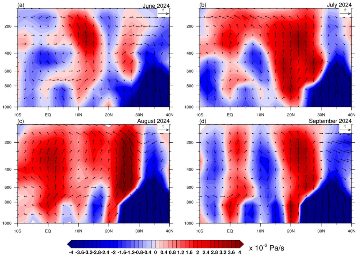
**Fig. 3.9: Latitude-Height Circulation Cross-section and Omega during a) June, b) July, c) August, and d) September 2024. Pressure vertical velocity (Omega) is shaded. The anomalies are averaged over longitudes 70°E-90°E.**
