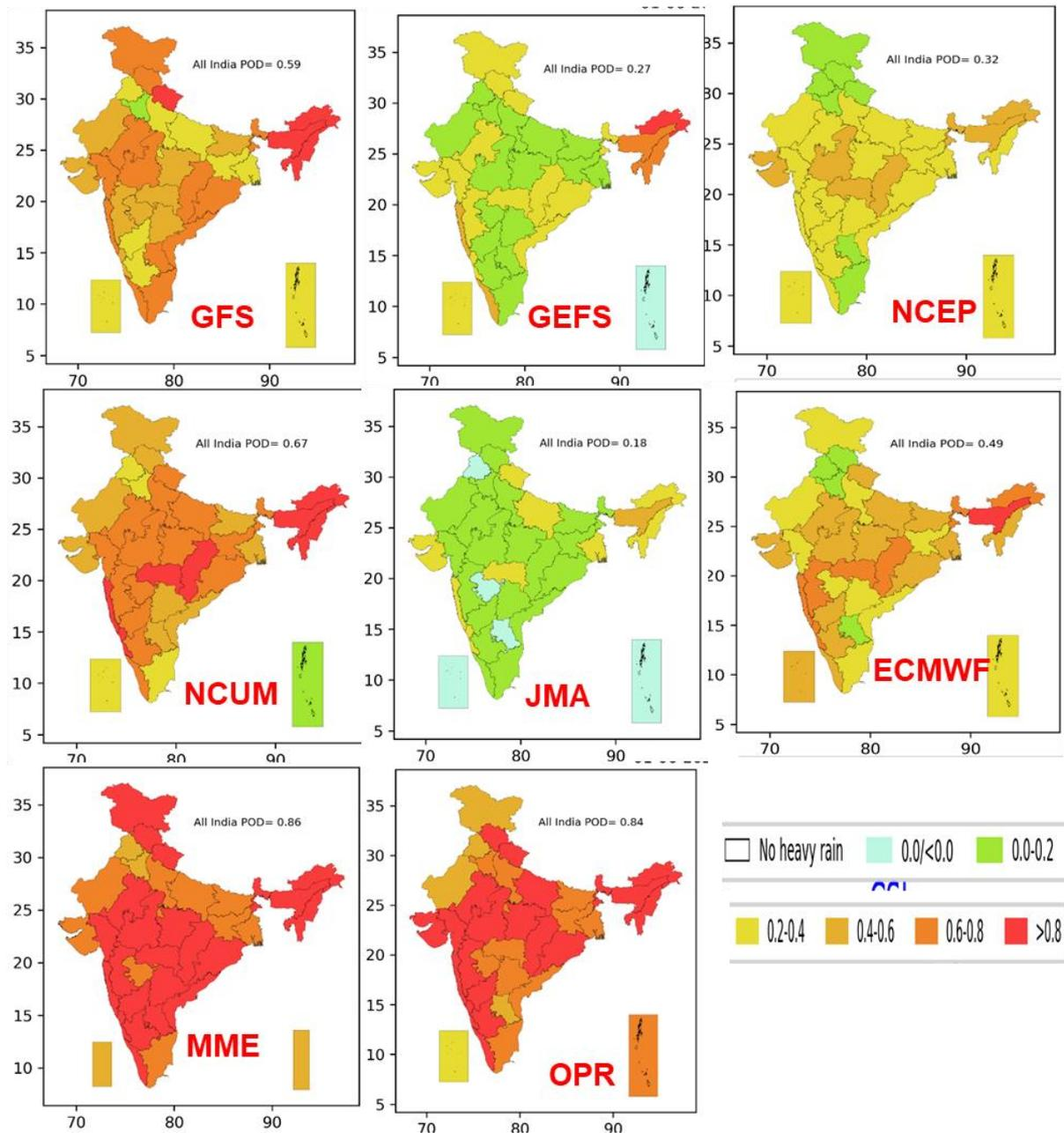
**Fig. 11.6: The POD of heavy rainfall ( $\geq 64.5$  mm) forecasts from various NWP models, MME, and OPR during the SW monsoon 2024 over different meteorological sub-divisions.**
