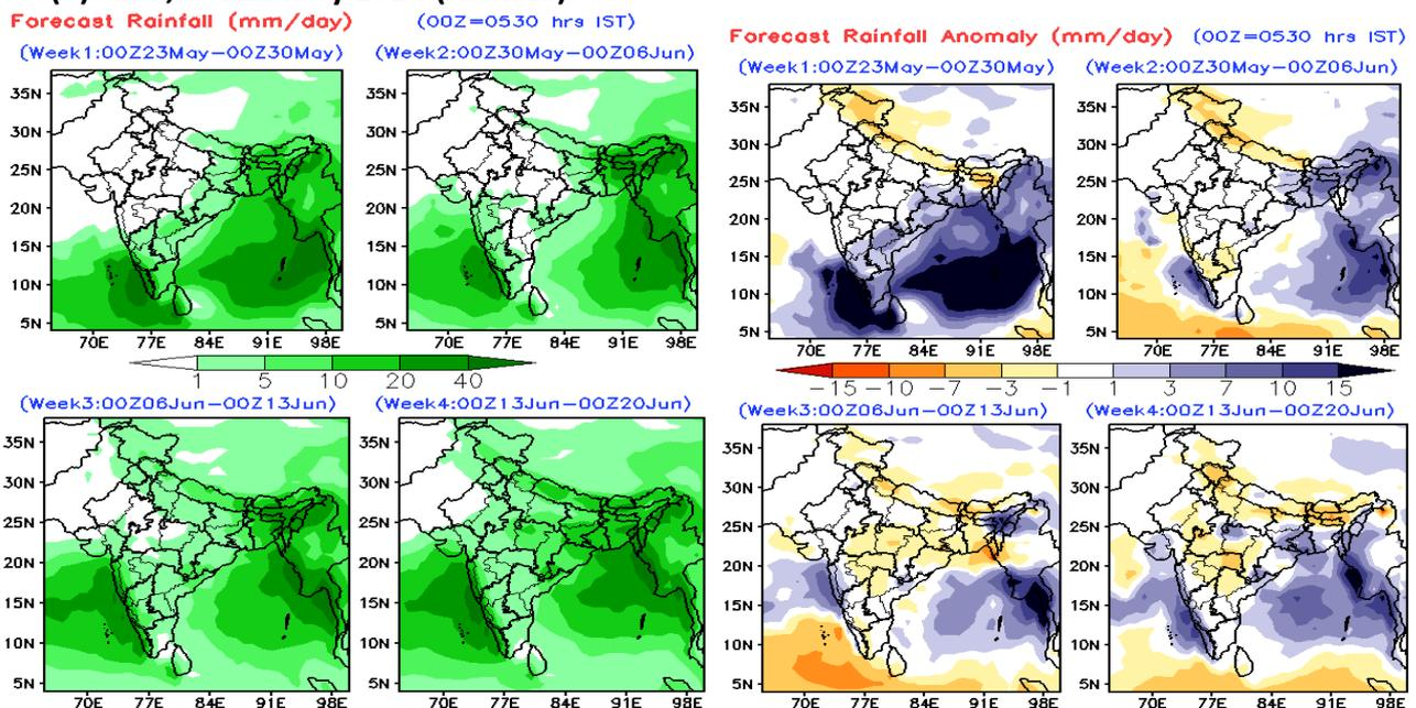
**Fig. 12.4:** (a) ERF 850 hPa mean wind and anomaly forecasts for four weeks valid for the period from 23 May to 20 June, 2024. (b) The corresponding mean and rainfall anomaly forecasts for 4 weeks valid for the period from 23 May to 20 June, 2024.
