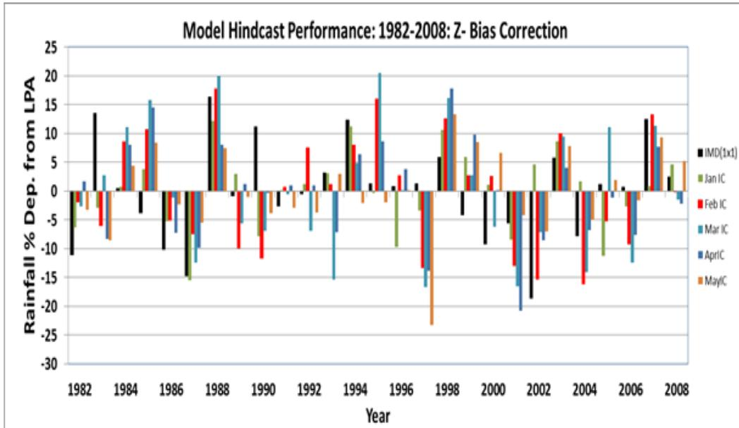
Fig.13.7: Performance of the model hindcast for the southwest monsoon season (June-September) rainfall over the country as a whole based on various initial conditions. The model hindcasts were bias corrected using the z-score transformation (correction for both mean and variance) method.
